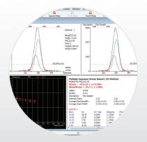
**PROTO XRDWIN 2.0.** An easy to use comprehensive Windows® based data collection and stress analysis package. Features include: linear and elliptical regression, Dolle-Hauk, and triaxial methods.
